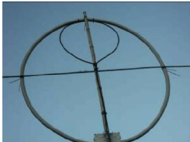
Figure 6 Coupling Loop on the Antenna Loop
