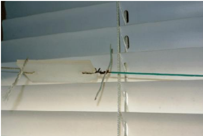
Picture 5 Capacitive Load at the Shortened Dipole Antenna for the 20- meter Band
