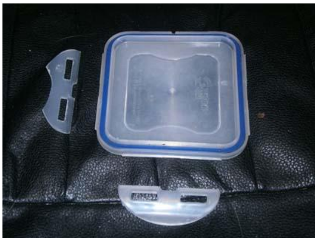
Picture 6 Cover with Cracked Retaining Tags
