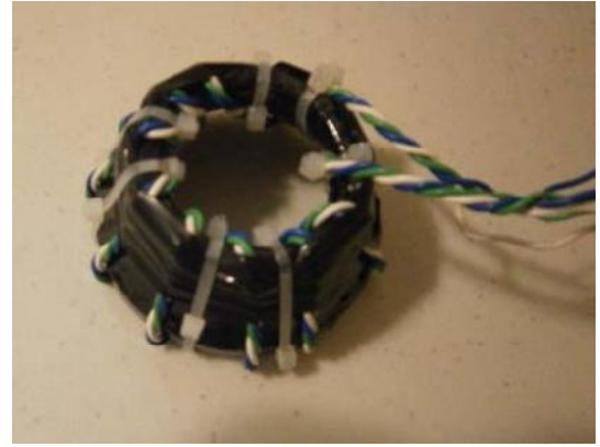
Figure 7 Unsymmetrical RF Transformer 1:9 on TV Yoke
