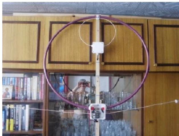
Picture 1 UA6AGW Antenna for 14 and 18- MHz Installed at my Room
