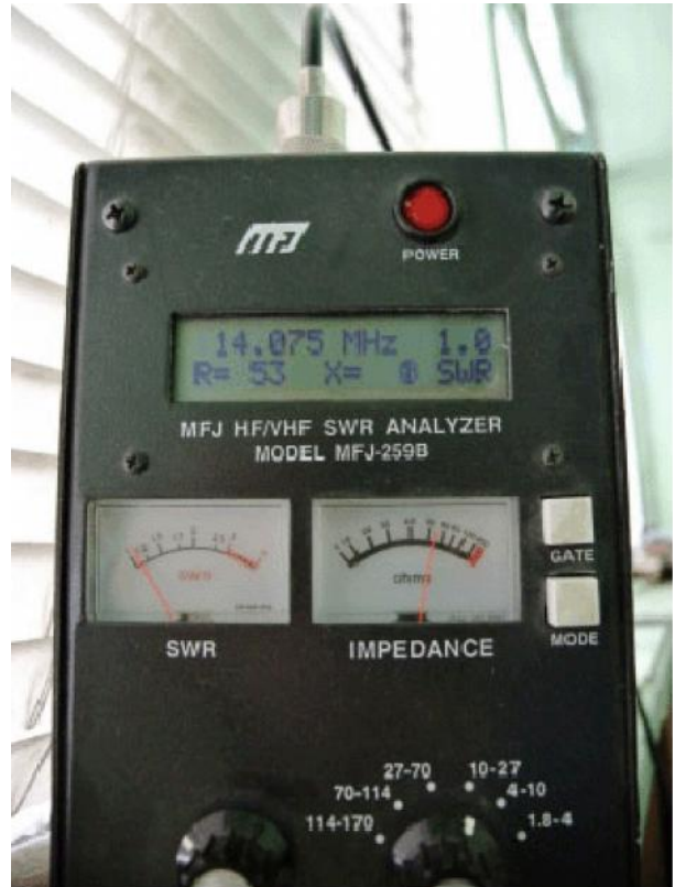
Picture 3 Antenna Analyzer MFJ- 259B Connected to the Tuned into Resonance Antenna
