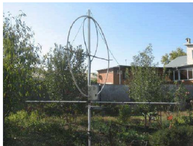
Picture 4 Coupling loop on the Directional UA6AGW Antenna V. 7.00
