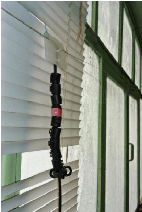
Picture 2 Shortened Dipole Antenna installed at my balcony
