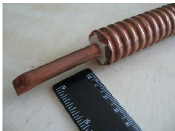
Figure 2 Coaxial cable "LCFS 114-50 JA, RFS (15239211)"
