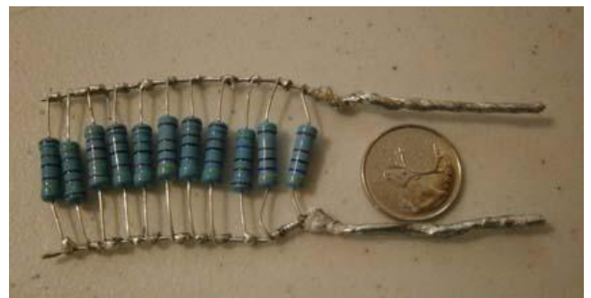
Figure 2 Practical Design of Home- Brew Termination Resistor
