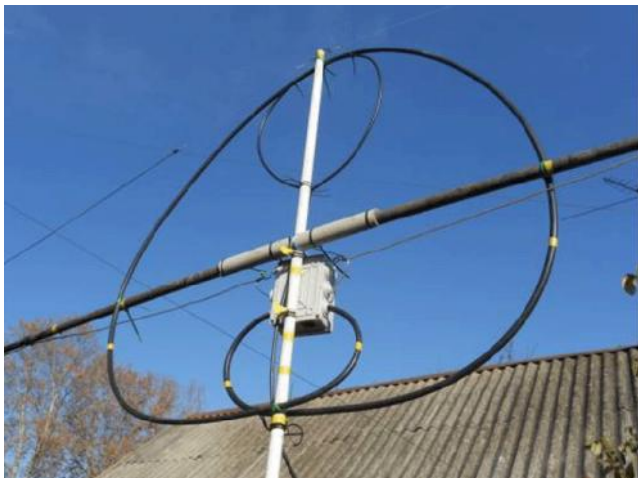
Picture 1 Loop of the UA6AGW Field Antenna V.40.21
