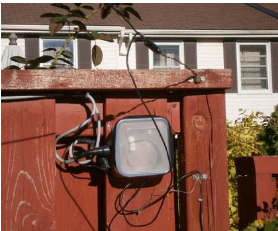
Picture 1 Feed Points of the Simple Broadband Antenna for the 40- meter Band
