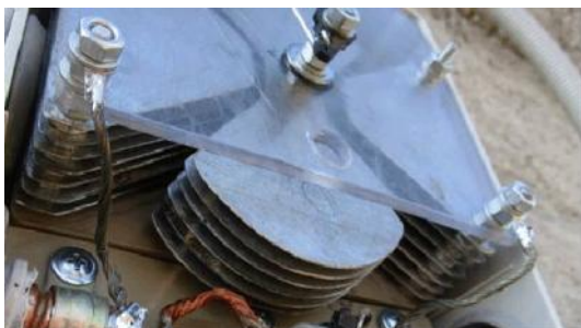
Figure 7 Capacitor of the UA6AGW Antenna V. 20-10.51
