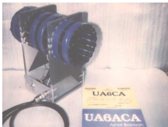
Figure 2 Picture of the Ferrite Magnet Antenna for the 160 and 80- meter Bands
