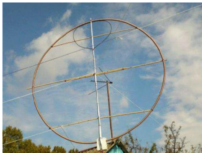
Figure 6 Picture of the UA6AGW Antenna for the 80-m Band
