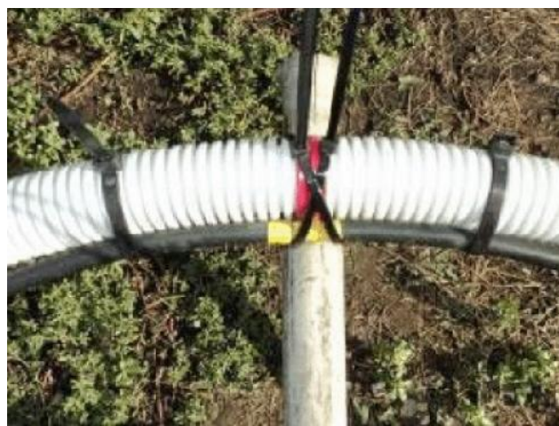
Figure 7 Bonding of the Coupling Loop to the Antenna Loop
