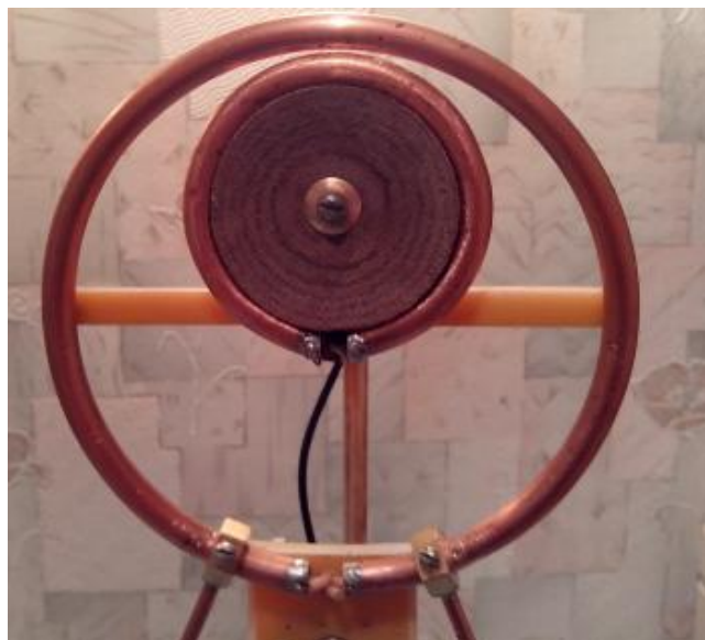
Figure 3 Coupling Loop at UA6AGW Antenna
