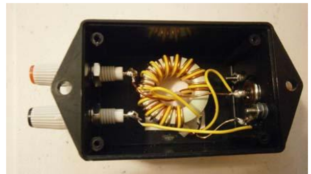
Figure 9 Unsymmetrical RF transformer 1:9 on the Base of Balun RBA- 1:1
