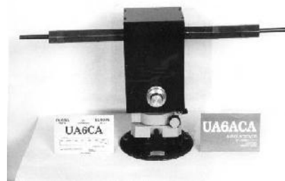
Figure 2 Ferrite Magnetic Antenna on the Revolving Stand
