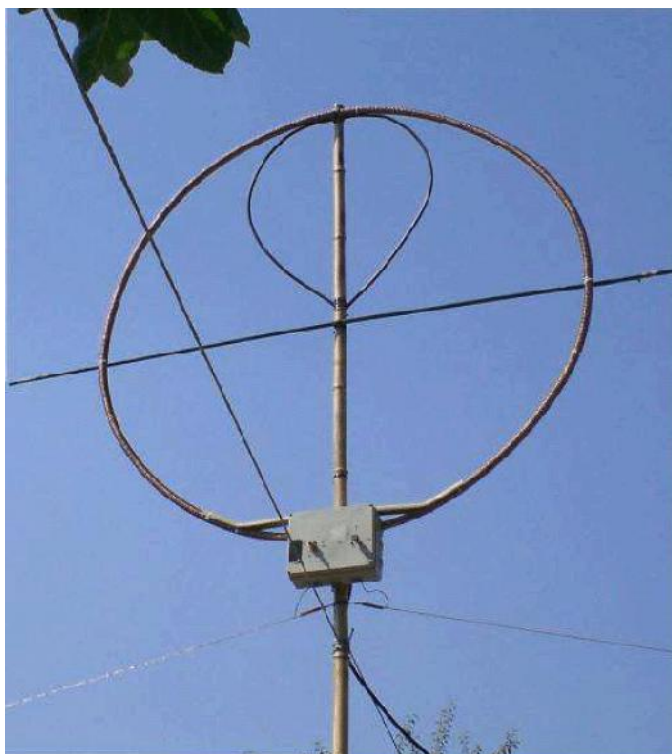
Figure 4 Picture of the UA6AGW Antenna for the 40-m Band
