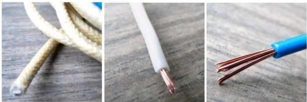
Photo 1 Examples of Some Good Antenna Strand Wires
