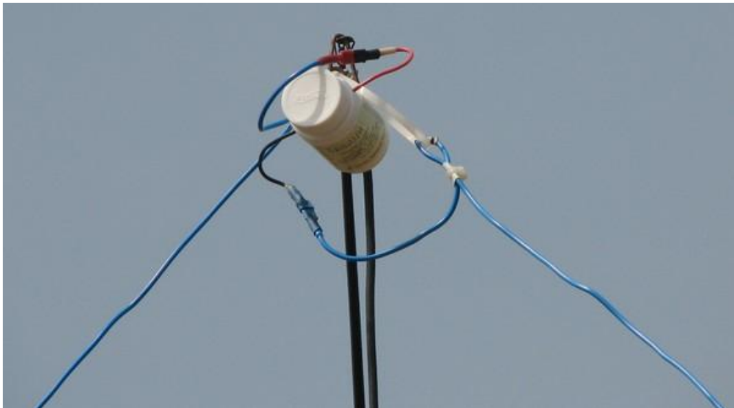
Matching Box on the Antenna
