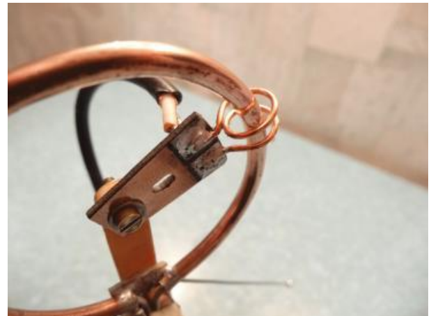
Figure 7 Fixture for Moving Coupling Loop
