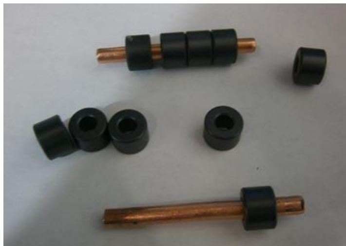
Ferrite Rings and Copper Tubes for the RF Transformer with Insulated Windings
