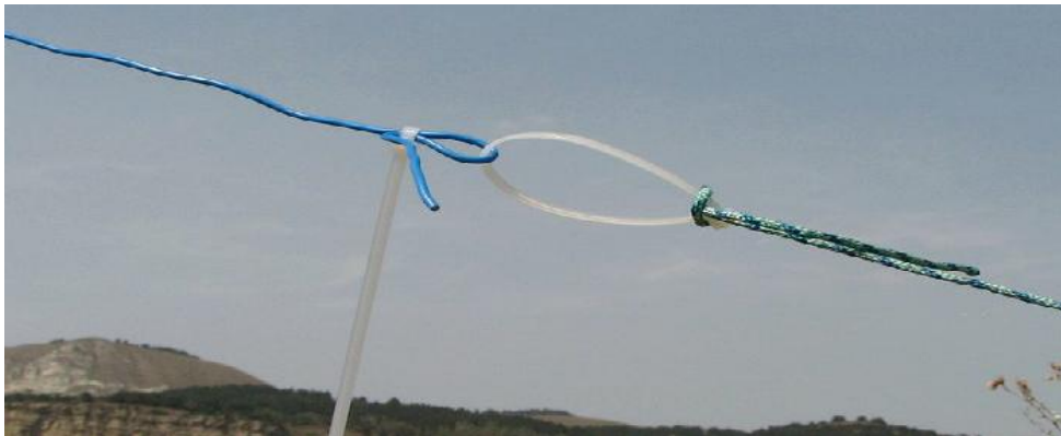
Antenna End Connection with a Guy
